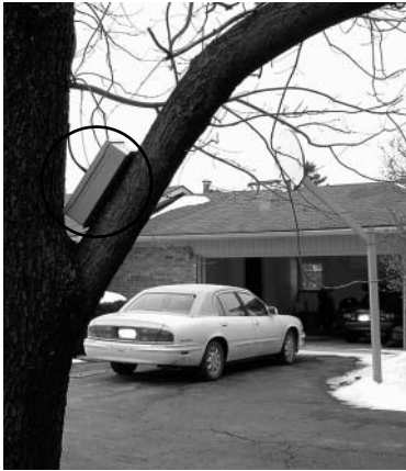
DA-611 installation illustration of the sensor buried under the drive and the receiver hidden in a nearby tree.
